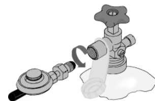
For POL cylinders, tighten counter-clockwise
