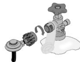
For Quick Connect cylinders, tighten clockwise
